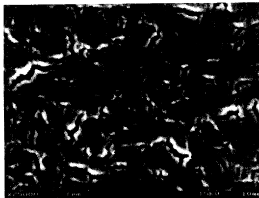
Fig. 3. An outer surface area of a peeled capillary, showing very big surface defects. Sputtered sample, same magnification as Fig. 1.
