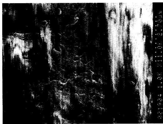
Fig. 14. Protein adsorption on inner capillary wall. Sample not covered by a gold layer (compare the contrast to Figs. 11–13 which were sputtered before).
